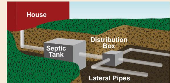
*Septic tanks are designed to allow bacteria and enzymes to biodegrade organic waste. This amazing process actually converts waste into water, carbon dioxide and small amounts of mineral matter!*
